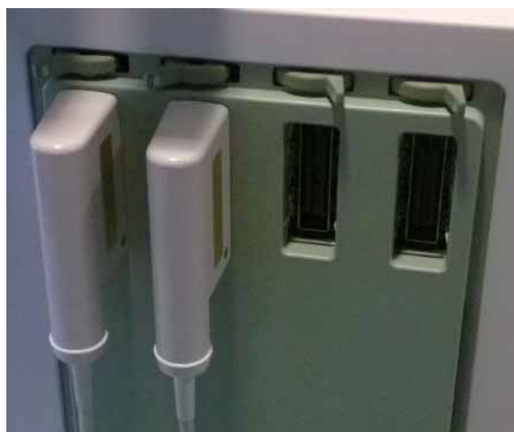
Figure 2-2. Transducer plugs and sockets.
